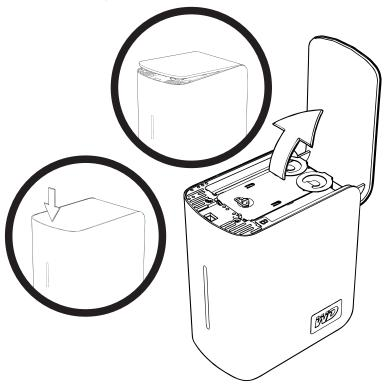
3. Loosen the thumbscrew that secures the drive cover plate. Remove the drive cover plate and set aside.
